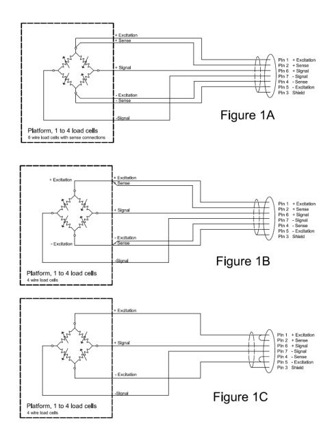
GK-Plus model must use the 6 wire connection and has certain limitations for wire size and length. Refer to the Approval Test Certificate for details.
