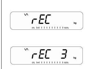
If you wish to recall any of the pre-stored limits, press [Tare] when "rECALL" is displayed. The display shows "rEC". Enter the number corresponding to the desired memory location (0 to 9) to be recalled. "rEC X" will be displayed for 2 seconds indicating the values stored in the location "X" is being recalled. The indicator will change to the recalled limits, weighing units and settings for the beeper and bar graph.
