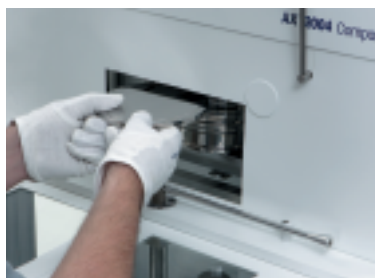
Manual dial weights for weighing range flexibility
