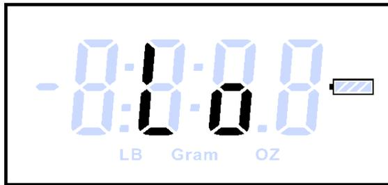
In this case, user will also see the empty battery icon blinking and once it appears, user should immediately replace the battery as the low battery condition is likely to degrade the weight measurement and giving a poor accuracy.
