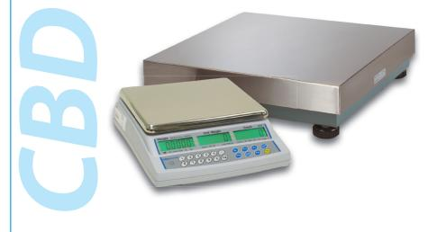
The CBD is a truly powerful counting scale that is fully capable of powering a remote base with up to four loadcells. Use the local scale to more accurately weigh the sample, then connect to the remote to weigh bulk items.
