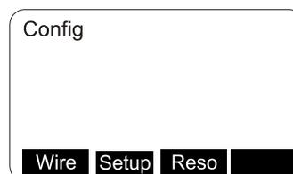
4. The unit is now in the Configuration mode. To see the rest of the softkeys available in this mode, press the **Right Arrow** key. All the Config softkeys are shown below.
