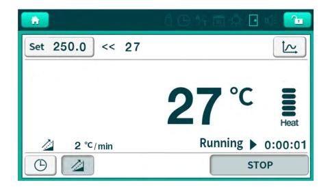
(2) Once you press the start button, the heating operation will be started, and you will see the temperature ramping rate is being applied in real time at the top left.
