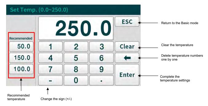
(2) When you enter the temperature settings, press the keypad to change the temperature value of the desired temperature. Press Enter to return to the basic mode. (If you press the ESC button without pressing Enter, the temperature settings will be canceled.)
