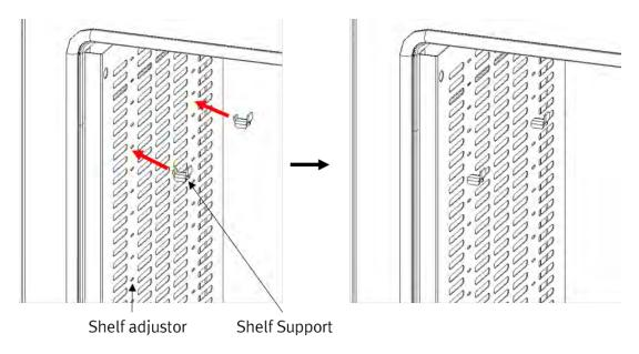
Place the shelf on the shelf support attached to the shelf adjustor. Depending on the model, up to 4 to 9 shelves can be installed.
