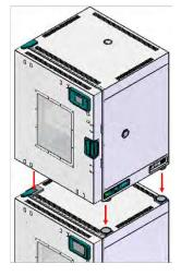
(4) After inserting the housing panel from the front, attach the rear bracket 2 using an M4x8 truss bolt.
