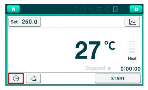
(1) Move to Timer Settings by pressing the button, in the Basic Mode.
