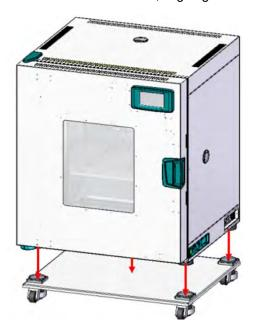
(2) Attach the rear Bracket1 and the housing panel to the bottom product using M4x8 Truss bolts.
