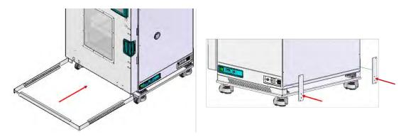
(3) Attach bracket 1 to the lower product with an M4x20 truss bolt using a power drill torque 1. Insert bracket 2 into the hinge and load the product according to the position.
