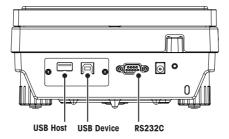
Interfaces and possible connectivity of peripheral devices:
