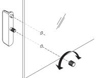
It is possible to remove the sliding glass doors for cleaning or for replacing. In this case you have to remove the handle first. Installing the handle after insertion of the glass door.
