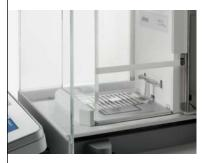
The SmartGrid weighing pan significantly reduces the effects of air turbulence on the weighing cell. Stabilization time is reduced and results are faster—particularly beneficial when working in a fume cupboard.
