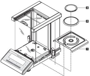
Push the side glass doors back as far as will go and place the following components on the balance in the specified order:
