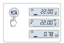
The « key can be used at any time to toggle between weight unit "UNIT 1", "RECALL" value (if selected) and weight unit "UNIT 2" (if different from weight unit 1) and the application unit (if any).
