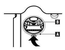
So that weighings can be carried out below the working surface (below-the-balance weighing), your balance is provided with a special hanger.
