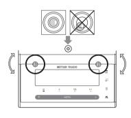
The balance has a level indicator and two adjustable leveling feet to compensate for slight irregularities in the surface of the weighing bench. The balance is exactly horizontal when the air bubble is in the middle of the level glass.
