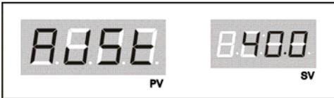
PV is put on the SV display and can be set as exactly as shown on thermometer. Set the value by pressing ▲ and ▼ , and conclude the setting by pressing
