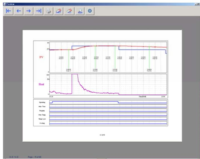
In case Print at equal intervals is ticked, PV and SV is printed in a regular interval(see above)
