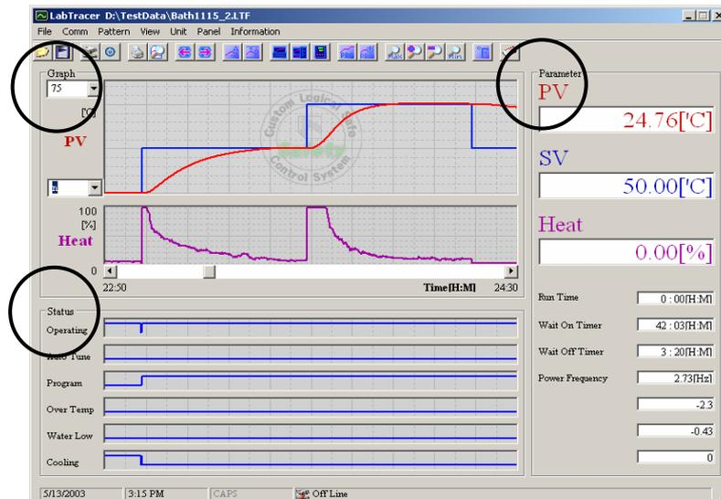
User can monitor operating process through three divided interfaces. (Graph, Parameter, Status)
