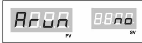
(1) This is selection of unit state after power failure. If you set yes the unit will run or else the unit will not run after power failure situation finished.
