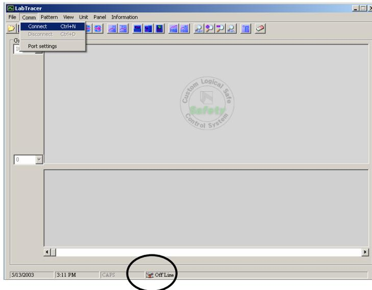
“On Line” displays on the bottom of the software, once communication is connected successfully. The window consists of 2 separate windows. Window on the top displays Temperature set point and actual temperature and window on the bottom displays output value of heating in graph mode.
