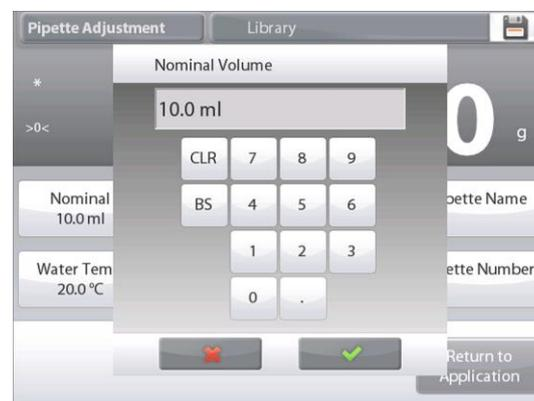
To adjust the water temperature, touch the **Water Temp** button.
