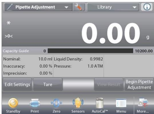
Touch **Begin Pipette Adjustment**. Follow the screen instructions, to **Place container on the pan**. Then **Press Tare**.
