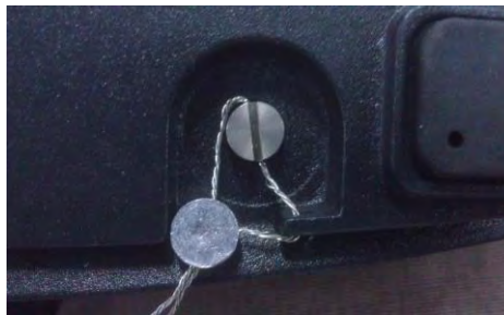
Locked with Wire Seal
