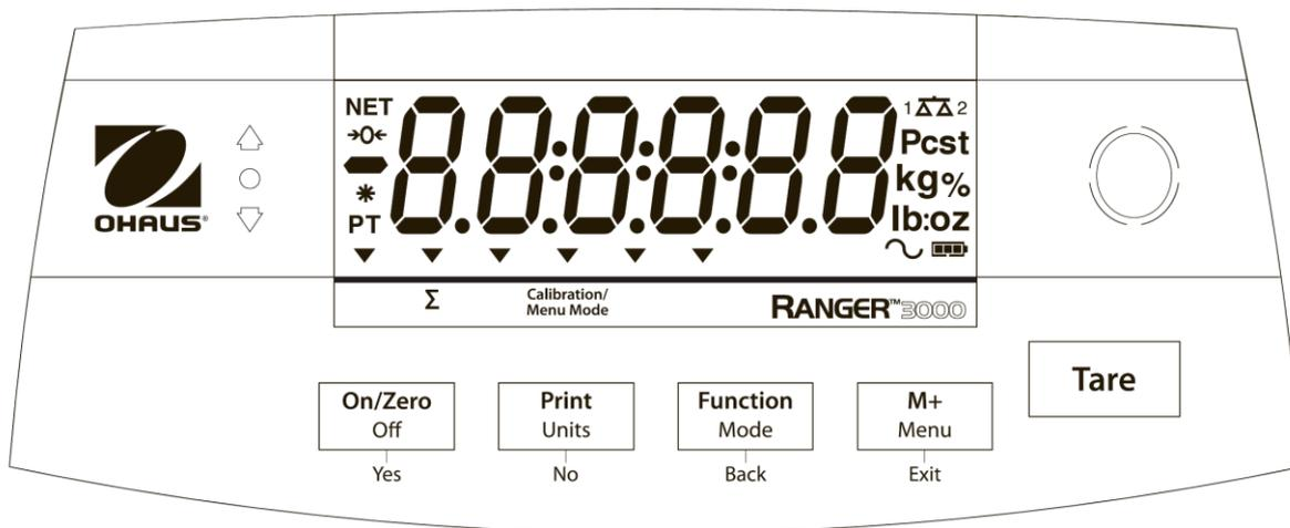
Figure 3-1. Ranger 3000 Control Panel with LCD display
