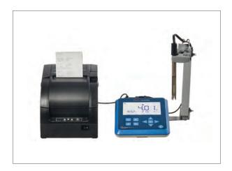
Data logs and calibration logs can be exported via the communication port to a computer or printer.
