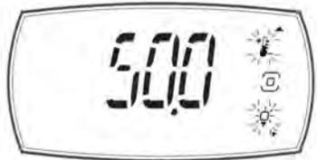
6. Press PRG to display the first menu item: St (=setpoint). Press PRG to display the parameter value;
