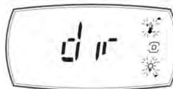
4. Press PRG to enter programming mode; the UP and DOWN buttons will flash and the first category of parameters dir (=direct functions) will be displayed;
