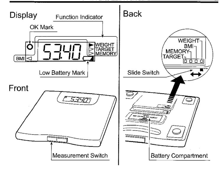
The following four measurements can be selected by the function switch.
